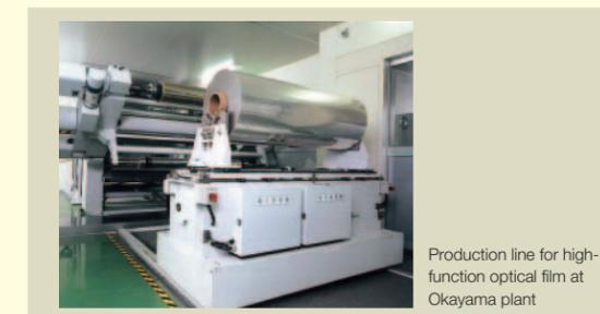
Production line for high-function optical film at Okayama plant
